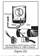
The sensor converts the air flow into a DC voltage, low frequency or high frequency signal. The Meter can only be used to test a DC voltage or low frequency signal.
